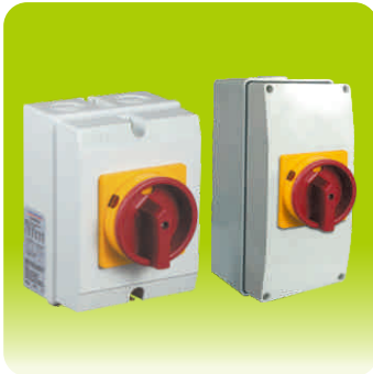
Part No.:DXWPIS/4P A true enclosed non-polarised DC switch 600V–1500V DC Max capable of delivering 6KA Ip66 rated
